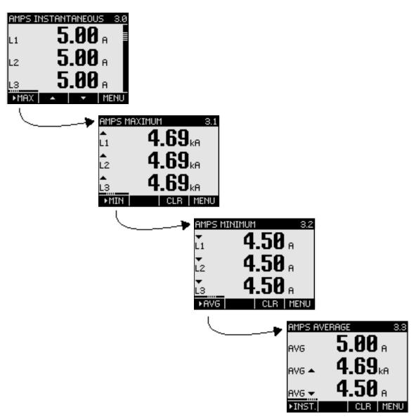
Figure 8-12 Display the instantaneous, maximum/minimum or average value
