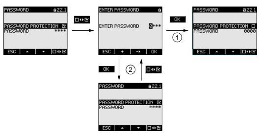
Figure 9-25 Switch off password protection
