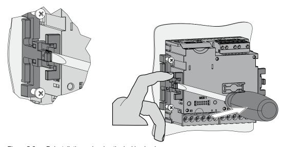
Figure 5-2 Deinstallation, releasing the locking hooks
