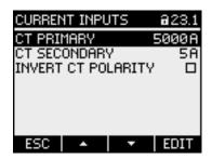
Figure 7-10 Device setting "CURRENT INPUTS - CT PRIMARY?"
