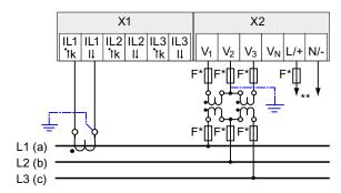
Figure 6-17 Connection type 3P3WB, with voltage transformer, with one current transformer
