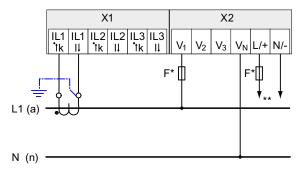
Figure 6-19 Connection type 1P2W, without voltage transformer, with one current transformer
