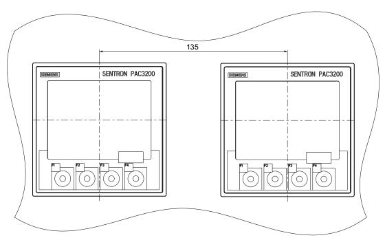
Figure 12-4 Side-by-side installation
