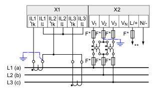
Figure 6-15 Connection type 3P3W, with voltage transformer, with two current transformers
