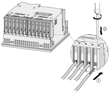
Figure 6-6 Connecting cables to the screw terminal
