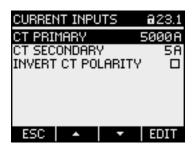
Figure 9-6 "CURRENT INPUTS" device setting
