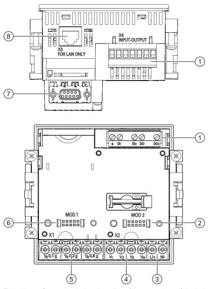
Figure 6-1 Connection designations, view of the rear and top of the device with screw terminals
