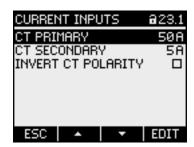
Figure 7-9 "CURRENT INPUTS" device setting
