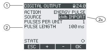
Figure 8-11 Edit mode of the device settings
