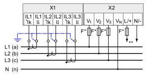
Figure 6-8 Connection type 3P4W, without voltage transformer, with three current transformers
