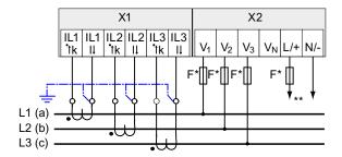
Figure 6-12 Connection type 3P3W, without voltage transformer, with three current transformers
