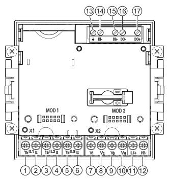
Figure 6-3 Terminal labeling with screw terminals
