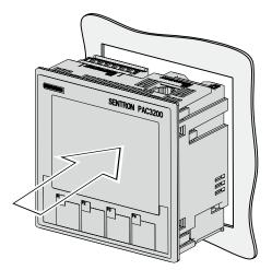
Installation step A, device with screw terminals
