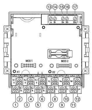
Figure 6-4 Labeling of the ring lug terminals
