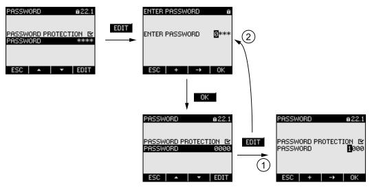
Figure 9-27 Change password - Password protection on
